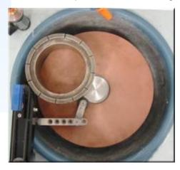
**Figure 1:** Image showing the Model 92002 Workstation with a diamondconditioning ring. The ring is used for removing material from the lapping plate surface to create a flat surface for lapping processes.
